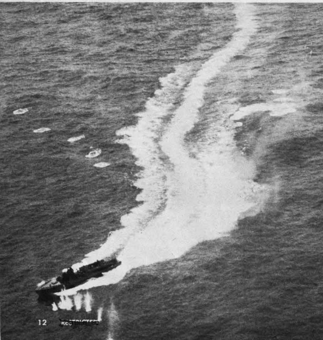
Simple, flat-sided hull of new type of Jap PT is seen in these overhead views. Depth charges are carried on the stern. Torpedoes, usually two, lie in tubes at each side. Picture below shows the straight bow railing, which is a recognition feature. U. S. railings are curved.
